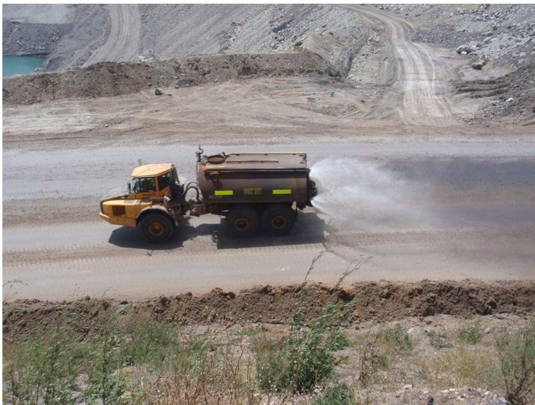
Figure 3: 30,000L Volvo Wobbly Water cart in operations at Werris Creek
